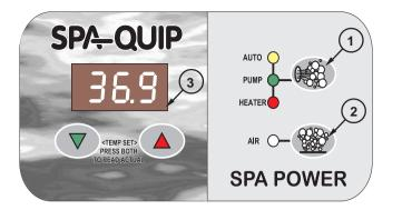
The Pump Mode button allows the user to switch the pump on or off as desired when using the pool. For safety the heater is always automatically controlled. Automatic operation is the default and the system returns to automatic mode by itself at a fixed time (96 minutes) after the user last pushed the purp button. Pushing the pump mode buttor then switches the pump on and terminates automate mode. If the pump was already on in automate then it will stay on.
